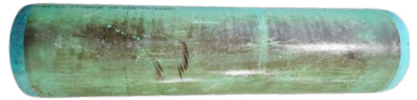
Figure 1: Sunburned AWWA C900 IB DR25 Pipe
