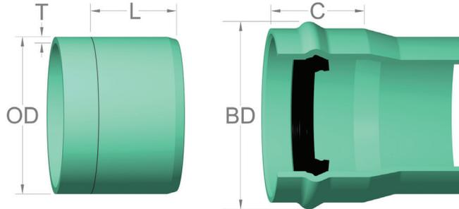
TUYAUX D'ÉGOUT AVEC JOINT D'ÉTANCHÉITÉ DIMENSIONS ET PERFORMANCES
