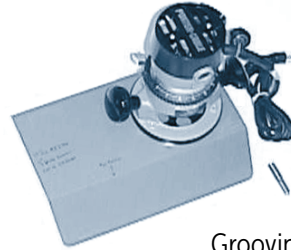
Grooving Jig with Router
