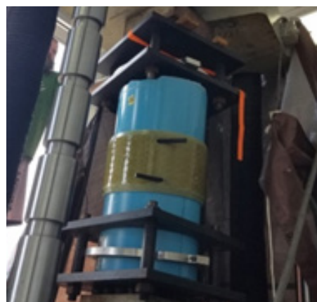
Certa-Lok Coupling Test Setup – Post Failure
