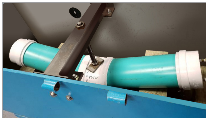
Figure 3 – Example of Angular Joint Deflection Setup for Pressure and Vacuum Tests for standard sewer fitting
